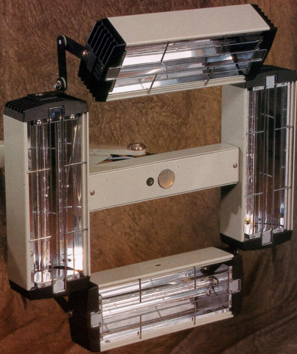
The Spectratek curing system's heating units consist of a tungsten filament high-temperature, halogen-filled quartz lamp that is encased in an aluminum cassette head with a high precision thermal reflector
